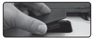
After the install is complete, snap the stake pocket covers into the stake pocket holes.
