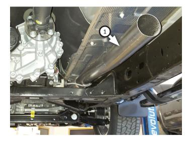
8. Place clamp (7) onto intermediate pipe (2) then connect it to inlet pipe with bend oriented upwards. Insert wire hanger into isolator and tighten clamp enough to allow for adjustment.
