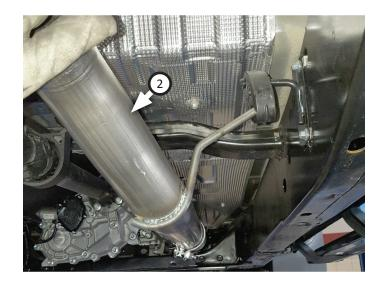
9. Place clamp (7) onto muffler (3) then connect it to intermediate pipe. Tighten clamp just enough to allow for adjustment then place clamp (7) onto muffler outlet.
