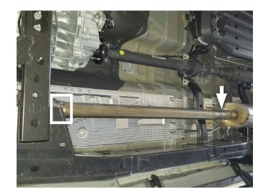
4. Support muffler and disassemble wire hangers from isolators. Remove tailpipe section from vehicle and set it aside.
